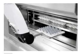
Robotic system for the loading vials in Nest.
