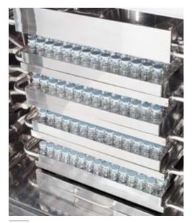
Vial batch ready for freeze drying.
